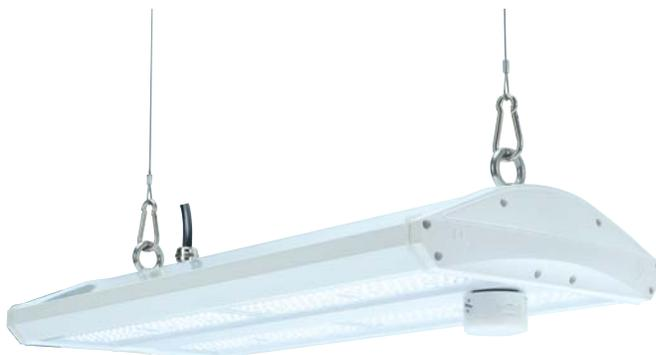
CPS NSF rated linear high bay series that covers food zone, splash zone, and non-food zones. UL listed and DLC listed (160W & 300W only on DLC). Smooth surface for easy cleaning. IP69K rated, 1500PSI hose spray.
